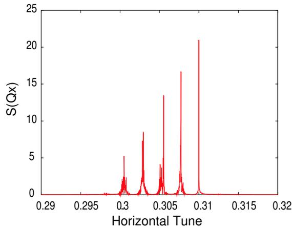
Figure 5: Head-on collisions in IPs 1, 2, 5 and 8. Phase advance symmetry restored between IP1 and IP5 and adjusted between 2 and 8.
