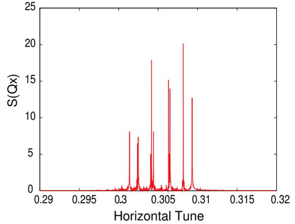
Figure 4: Head-on collisions in IPs 1, 2, 5 and 8 with nominal LHC phase advance between interaction points.
