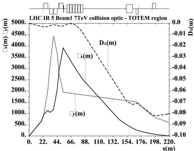
Figure 2: Nominal optics from the IP of CMS to the Roman Pot at 220 m.
