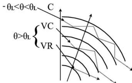
Figure 4: Scheme of a bent crystal.
