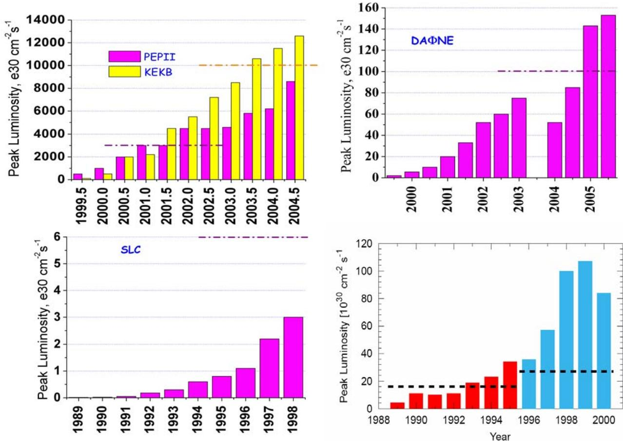
Fig.3: Luminosity of e+e- colliders: PEP-II and KEK-B, DAFNE, SLC and LEP.
