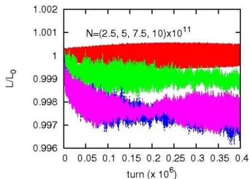
Figure 4: Luminosity evolution versus intensity for a Piwinski angle of 3.5, H-H crossing and several bunch charges
