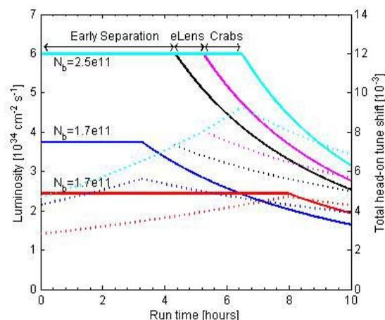
Figure 3: Luminosity with levelling and HV crossings versus time: 1)  $N_b=1.7 \cdot 10^{11}$  ppb, 2)  $N_b=2.5 \cdot 10^{11}$  ppb.
