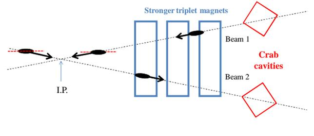
Figure 2: Interaction region for the Full Crab Crossing (FCC) scheme with very small  $\beta^*$  (8 cm) and crab cavities for tilting the bunches.
