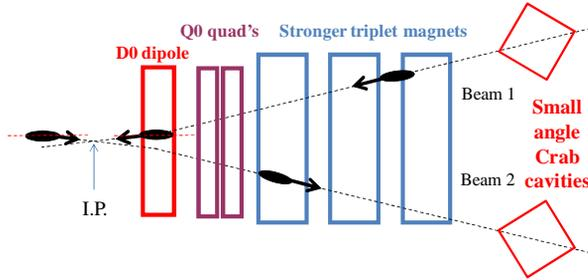
Figure 1: Interaction region for the Early Separation (ES) scheme with very small  $\beta^*$  (8 cm) and early separation dipoles D0 close to the interaction region.
