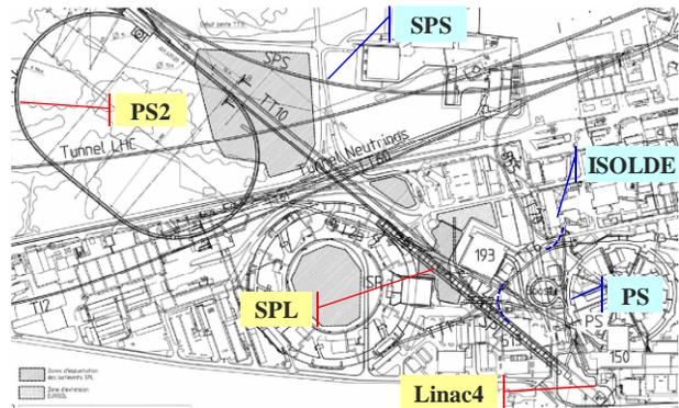
Figure 7: Layout of the new injector complex.
