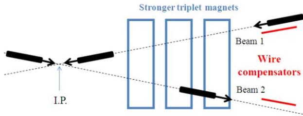
Figure 3: Interaction region for the Large Piwinski Angle (LPA) scheme with moderate  $\beta^*$  (25 cm) and wire compensators against long range beam-beam effects.
