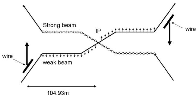
Figure 1: The compensation wires will be positioned 104.93m from IP1 and IP5, where the beams are already in their separated beam-pipes [1]. The arrows indicate the strength and direction of the force due to the LR-BB and the wire. The two wires shown compensate the force exerted by one ‘strong’ beam on the other ‘weak’ beam. The equivalent set of two wire compensators will be installed for the second beam, for which the roles of strong and weak beam are interchanged.
