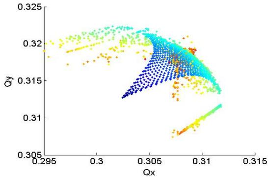
Figure 9: Tune footprint of LR and HO – collision.
