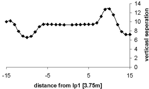
Figure 2: The beam-beam separation varies between  $7\sigma$  and  $13\sigma$ . This variation is one of the reasons why the compensation with a single wire cannot work perfectly.
