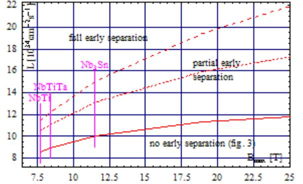
Figure 4: Luminosity [ $10^{34} \text{ cm}^{-2} \text{ s}^{-1}$ ] enhanced by early separation versus operating field [T] for  $l^*=19 \text{ m}$ ,  $\phi_{\text{coil}}=100 \text{ mm}$  and ultimate beam current
