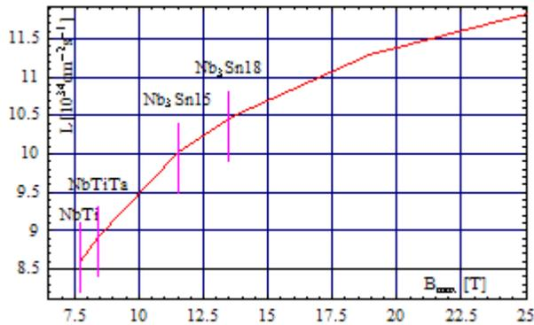
Figure 3: Luminosity [ $10^{34} \text{ cm}^{-2} \text{ s}^{-1}$ ] versus operating field [T] for  $l^*=19 \text{ m}$ ,  $\phi_{\text{coil}}=100 \text{ mm}$  and ultimate beam current; the index for Nb<sub>3</sub>Sn is the quench field.
