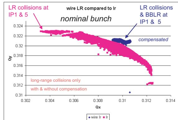
Figure 17: LHC tune footprint with only long-range collisions at IP1 and IP5 with and without wire compensation for a nominal bunch, computed by BBTRACK.
