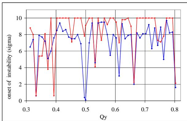
Figure 23: LHC tune scan for a nominal bunch. Shown is the dynamic aperture without (blue) and with wire compensation (red) as a function of the vertical tune, for a constant horizontal tune of  $Q_x = 0.31$ , computed by BBTRACK.
