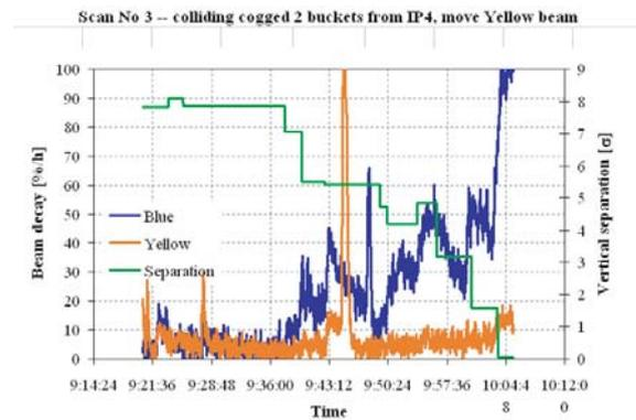
Figure 28: RHIC experiment on 28 April 2005, scan no. 3, two bunches collide 10.65 m from IP4; the yellow beam is moved vertically; the lifetime of both beams and their separation is shown as a function of time.
