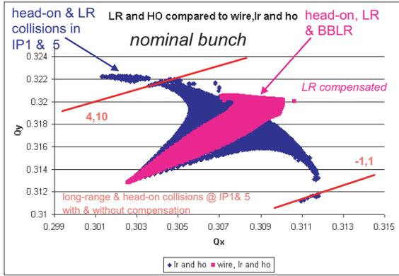
Figure 19: LHC tune footprint with long-range and head-on collisions at IP1 and IP5 with and without wire compensation for a nominal bunch, computed by BBTRACK.
