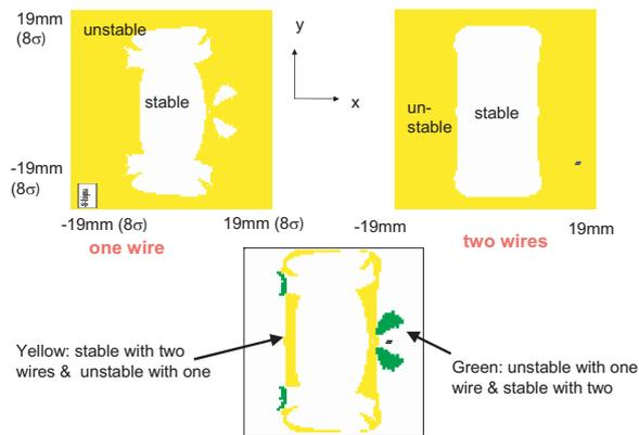
Figure 7: Simulated stability region in the  $x$ - $y$  plane for the SPS with one (top left) and two wires (top right), and the difference (bottom). The horizontal and vertical scales both extend over  $\pm 8\sigma$ . The wire current is 240 A and the horizontal beam-wire distance 19 mm. The simulation was performed with BBTRACK.
