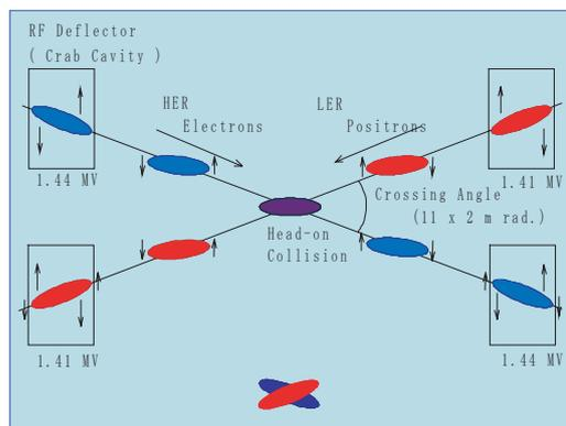
Figure 34: Schematic of crab crossing at SuperKEKB [32].
