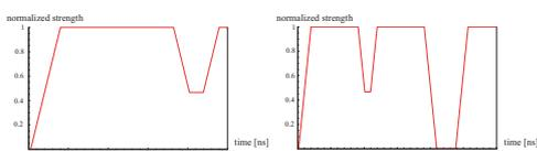
Figure 33: Examples of pulsed-wire excitation patterns for LHC (zoom).
