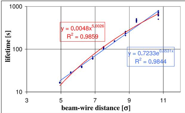
Figure 4: SPS beam lifetime measured as a function of the beam-wire distance, in an experiment conducted on 09/11/2004, with a single-wire excitation of 190 A, tunes  $Q_x = 0.3208$ ,  $Q_y = 0.2914$ , emittance  $\gamma\epsilon_x \approx \gamma\epsilon_y \approx 1.4 \mu\text{m}$ , and an rms beam size of about 1.56 mm. The beam was separated from the wire in the vertical direction.
