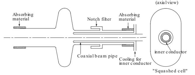
Figure 42: Schematic of squashed cell crab cavity for the KEKB B factory [35, 36].
