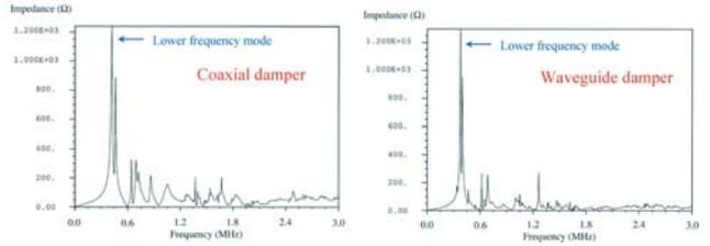
Figure 46: Longitudinal impedance of two low-impedance crab cavity designs for Super-KEKB with either coaxial damping (left) or waveguide damping (right) [46].
