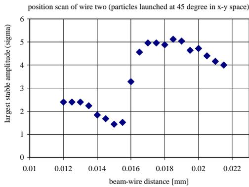
Figure 11: Maximum stable amplitude (dynamic aperture) as a function of the vertical position of the second wire simulated by the code BBTRACK. The distance of the first wire is held constant at 19 mm.
