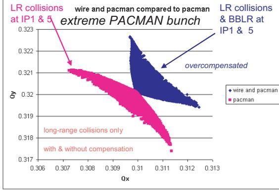
Figure 18: LHC tune footprint with only long-range collisions at IP1 and IP5 with and without wire compensation for an extreme PACMAN bunch, computed by BBTRACK.
