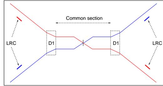
Figure 12: Schematic position of the long-range correctors at IP1 or IP5 of LHC [11].
