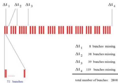
Figure 32: The nominal LHC filling pattern [1].
