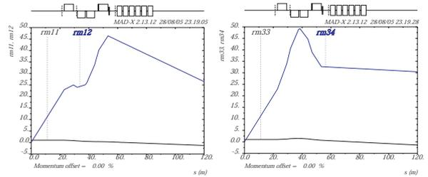
Figure 38: The horizontal matrix elements  $\tilde{R}_{12} = -R_{12}$  and  $\tilde{R}_{11} = R_{22}$  (left) and the vertical ones  $\tilde{R}_{34} = -R_{34}$  and  $\tilde{R}_{33} = R_{44}$  (right) from the IP to prospective crab-cavity locations.
