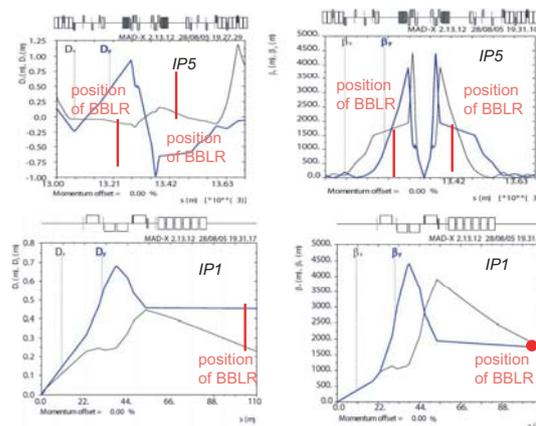
Figure 25: The LHC design dispersion (left) and beta functions (right) on either side of IP5 (top) and on the right side of IP1 (bottom). The foreseen position of the wire compensators is indicated by the vertical red lines or dot, respectively.
