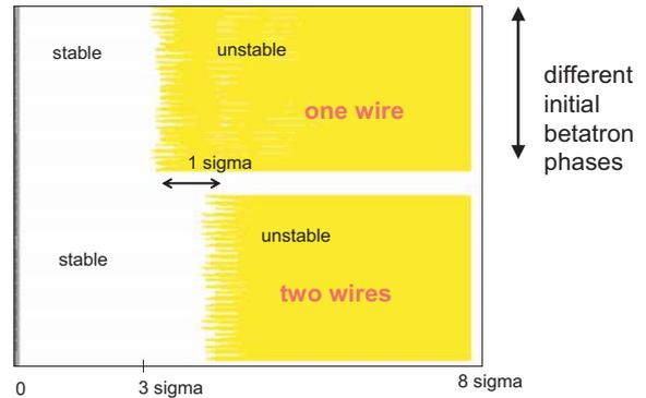
Figure 8: Simulated stability boundary (color) for the SPS as a function of horizontal starting amplitude (horizontal axis) for one (top) and two wires (bottom). The different rows refer to different initial betatron phases. The wire current is 240 A and the horizontal beam-wire distance 19 mm. The simulation was performed with BBTRACK.
