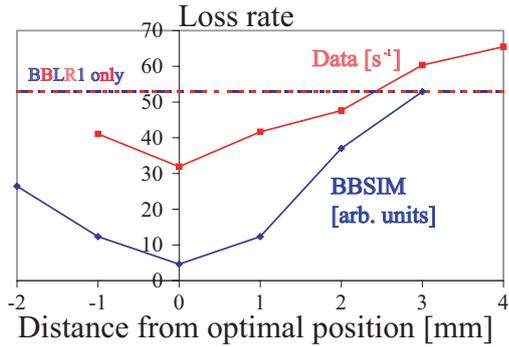
Figure 10: Relative SPS beam loss rate in  $s^{-1}$ , as measured over 2.4 s, and simulated loss rate in arbitrary units vs. the vertical position of the compensating second wire. Measured and simulated loss rates for a single wire are indicated by the two superimposed straight lines.
