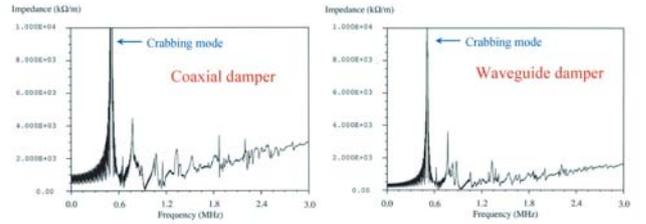
Figure 45: Horizontal impedance of two low-impedance crab cavity designs for Super-KEKB with either coaxial damping (left) or waveguide damping (right) [46].
