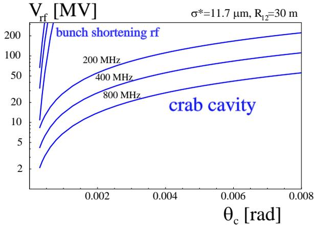
Figure 40: Zoom of Fig. 39 highlighting the crab-cavity voltage required for an LHC upgrade as a function of the full crossing angle, for different rf frequencies and longitudinal emittances. The curves are computed from Eqs. (7) and (8). An IP beam size of  $11.7 \mu\text{m}$  and  $R_{12} = 30 \text{ m}$  from the crab cavity to the IP are assumed.
