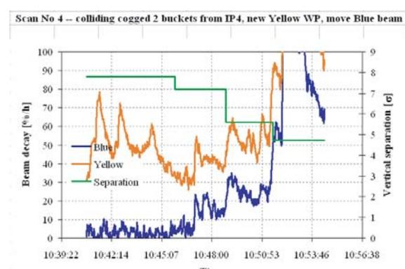
Figure 29: RHIC experiment on 28 April 2005, scan no. 4, two bunches collide 10.65 m from IP4; a new working point was chosen for the yellow beam; the blue beam is moved vertically; the lifetime of both beams and their separation is shown as a function of time.
