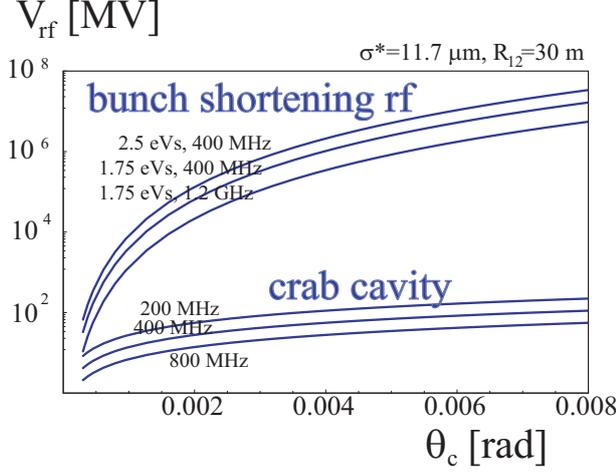
Figure 39: Bunch shortening rf voltage for  $R_{\Theta} = 0.68$  and crab-cavity voltage as a function of the full crossing angle, for different rf frequencies and longitudinal emittances. The curves are computed from Eqs. (7) and (8). An IP beam size of  $11.7 \mu\text{m}$  and  $R_{12} = 30 \text{ m}$  from the crab cavity to the IP are assumed.
