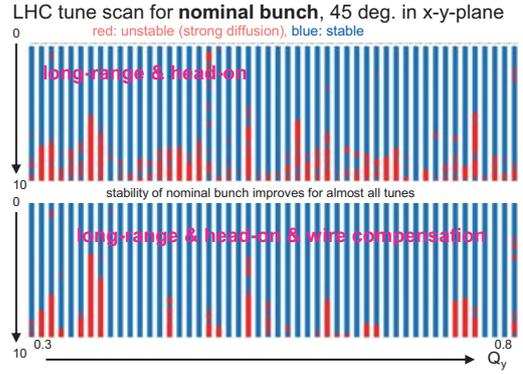
Figure 21: LHC tune scan for a nominal bunch. Shown are stable (blue) and unstable (red) start amplitudes in descending order without (top) and with wire compensation (bottom) as a function of the vertical tune, for a constant horizontal tune of  $Q_x = 0.31$ , computed by BBTRACK.
