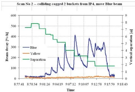
Figure 27: RHIC experiment on 28 April 2005, scan no. 2, two bunches collide 10.65 m from IP4; the blue beam is moved vertically; the lifetime of both beams and their separation is shown as a function of time.
