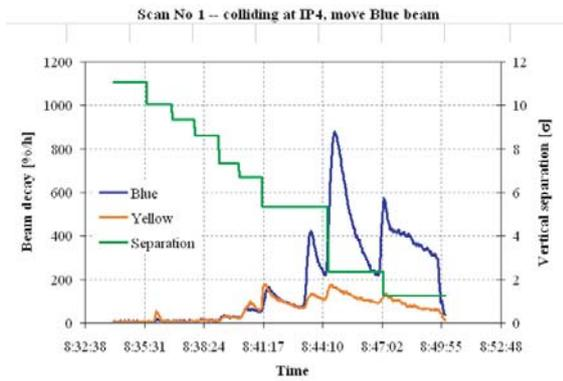
Figure 26: RHIC experiment on 28 April 2005, scan no. 1, two bunches collide at IP4; the blue beam is moved vertically; the lifetimes of both beams and their separation are shown as a function of time.
